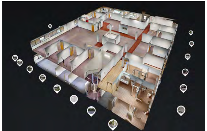
Matterport Scan of Existing Building
