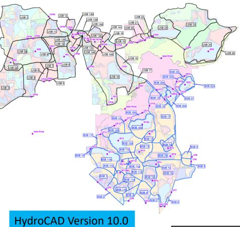
HydroCAD Version 10.0 was used for Pre- and Post- mining phase stormwater analysis
