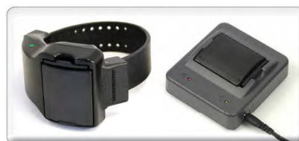
To the best of our knowledge, the BI LOC8 is the only GPS solution equipped with Wi-Fi location detection and a proximity sensor.
